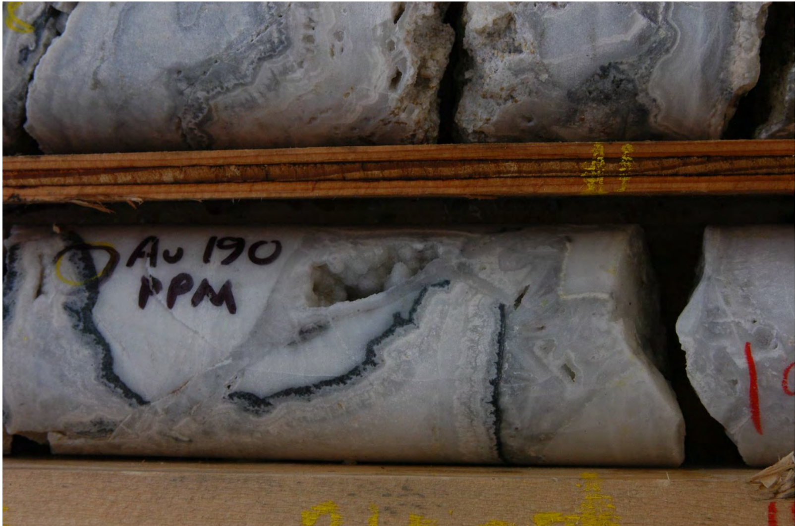
Banded quartz-adularia-ginguro. pXRF of ginguro returned 190ppm Au. Sample interval assayed 18.3 g/t Au and 119.0 g/t Ag over 1m (191-192m).
