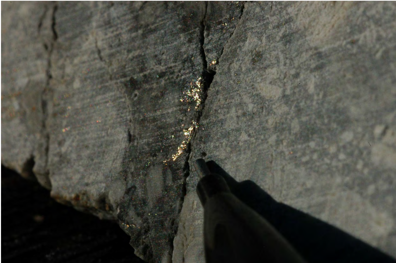
Visible gold in quartz veinlet (235.4m). Sample interval assayed 132 g/t Au and 127 g/t Ag over 0.5m (235.0-235.5m).
