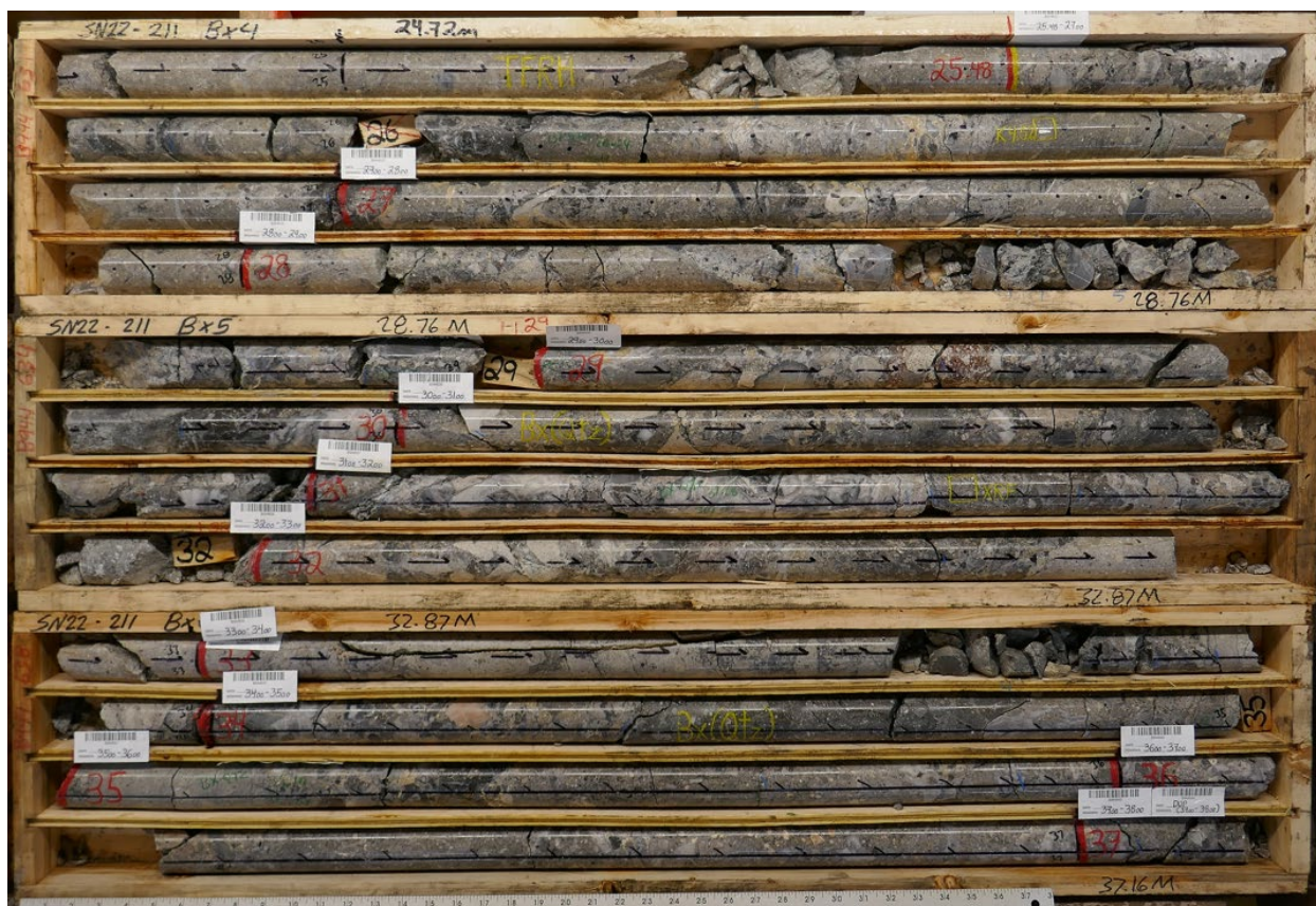
FIGURE 7.20 FMN HETEROLITHIC BRECCIA IN DRILL HOLE SN22-211 (24.72 M TO 37.16 M)
