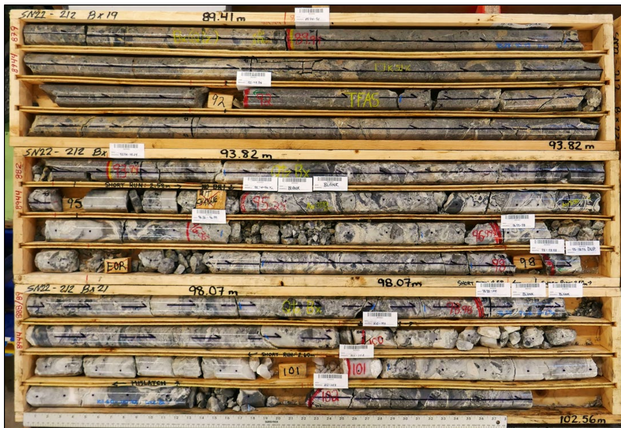
FIGURE 7.18 FMN VEIN ZONE 1A IN DRILL HOLE SN22-212 (89.41 M TO 102.56 M)
