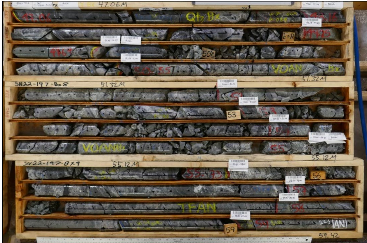
FIGURE 7.19 FMN VEIN ZONE 1B IN DRILL HOLE SN22-197 (47.06 M TO 59.42 M)
